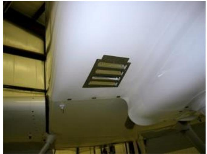
I also 'glassed a "lip" on the exhaust outlet portion of the cowl in order to provide a bit of a venturi effect to draw additional air out. Not sure how effective it is, but it does look better.
