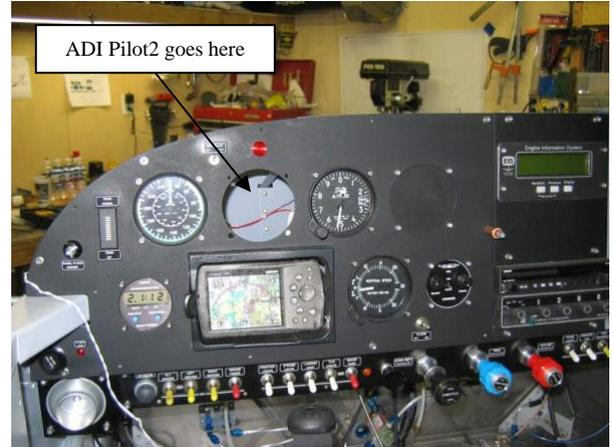
completion of may panel. I am waiting on TruTrak to deliver my ADI Pilot 2. This is a combination of their popular 2-axis autopilot and a solid-state gyro horizon in one small package. Wiring went well and may be my favorite construction task to date.
