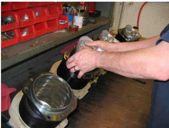
Next we got the pistons and rings assembled and mounted the cylinders on the case - lots of bolts and special torques here. Ryan just kept pulling parts off the cart and like magic, they fit. It was clear he had done this more than a few times. The clock and our stomachs told us it was lunchtime.
