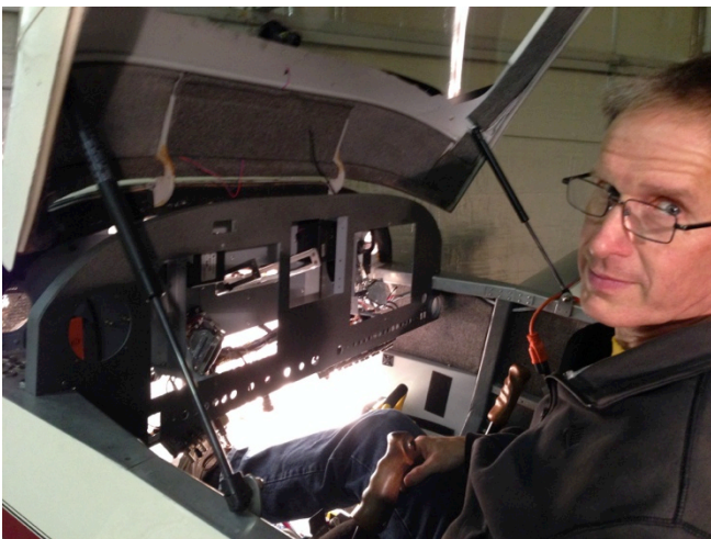
The old panel removed and starting to install the new parts.
