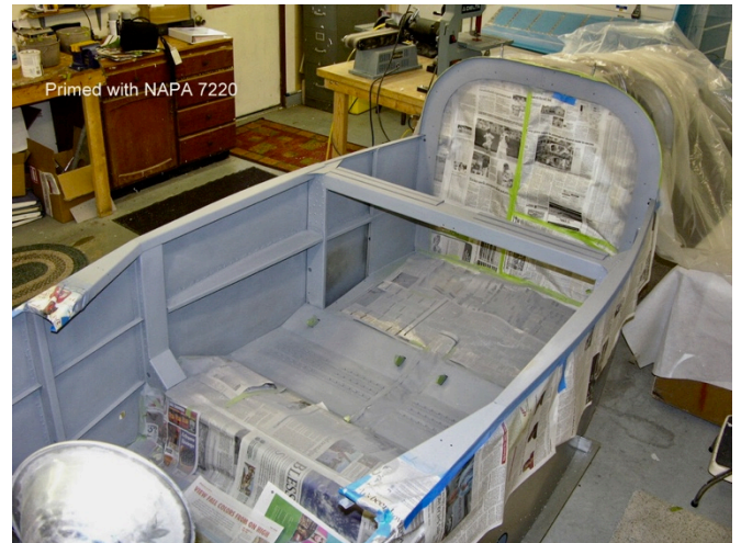
Sprayed with NAPA 7220 self-etching primer
