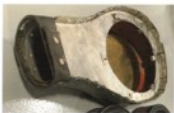
To see if the filter fits correctly, use a flashlight to look into the inlet. If it needs replacing, remove the bolts holding the airbox to the carburetor. A
