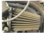
This air filter can be cleaned and oiled. Use the K&N filter recharger kit, part No. 08-00722 from Aircraft Spruce. The same kits can be found at most automotive stores.
