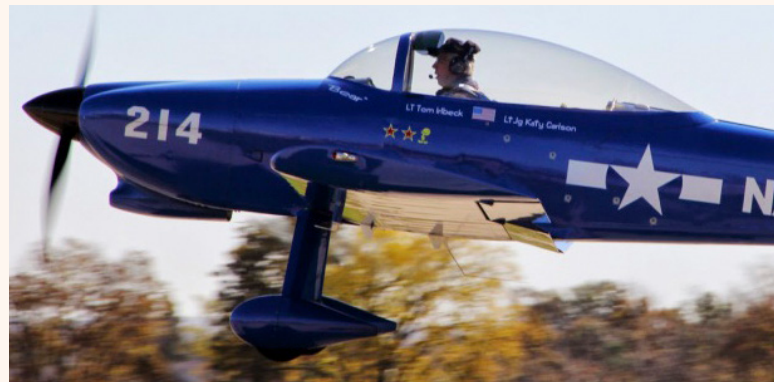
Tom Irlbeck built a RV-8 in his basement and painted it with the Navy colors and numbers which were the same as on the F-4 that he flew in Vietnam. 20,000 rivets in his home-built plane.
